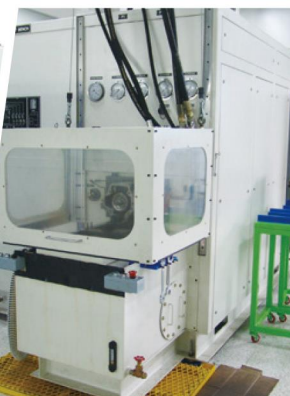
Pump Test Stnad
